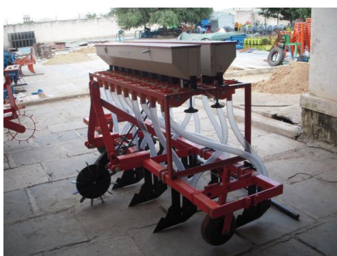
Zero till multi crop planter developed by M/s Varsha Associates
